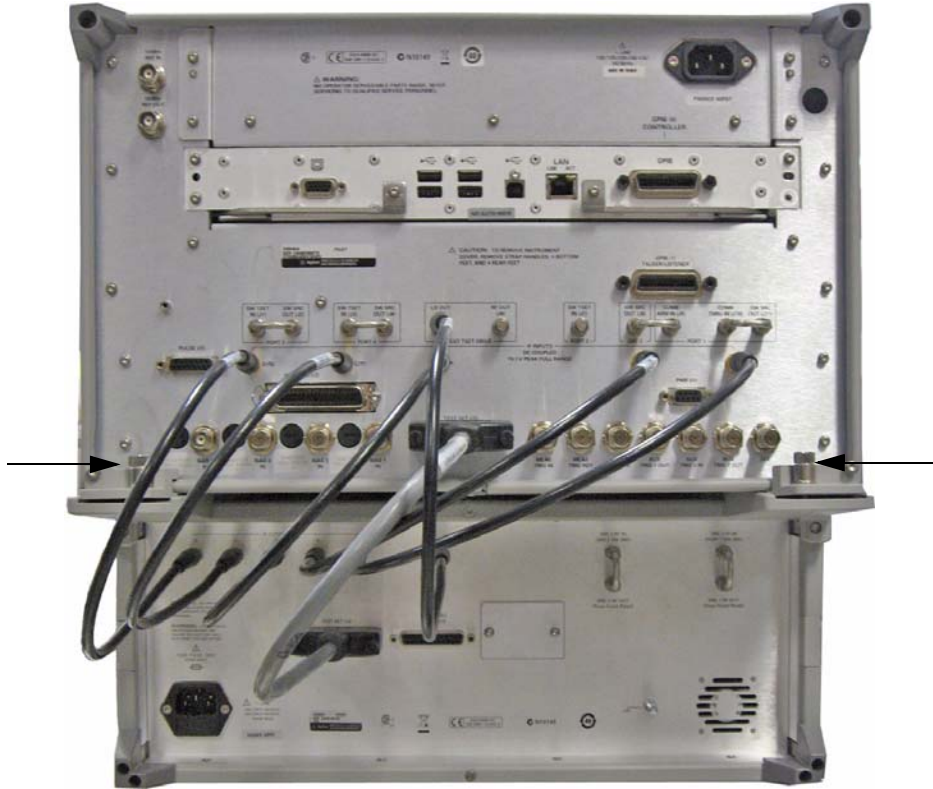
Figure 3-5 Locking Feet Screws
