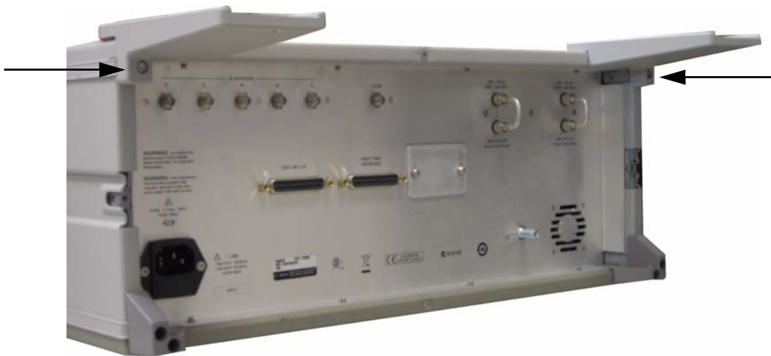
Figure 3-3 Install Locking Feet on N5261/62A
